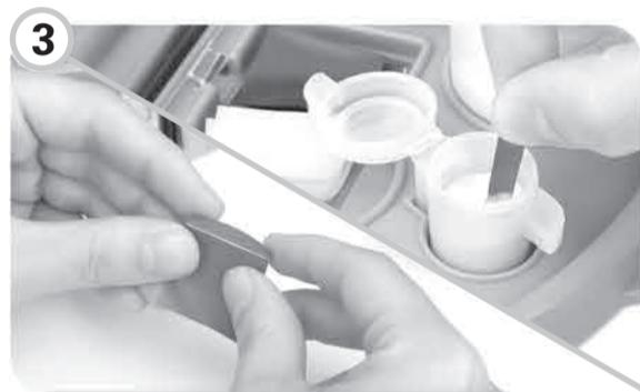
**NOTE:** Each color square has 5 peelable mini-strips. Fold strip on perforated line, then peel from backing. Push strips down into base paint & cover completely.
